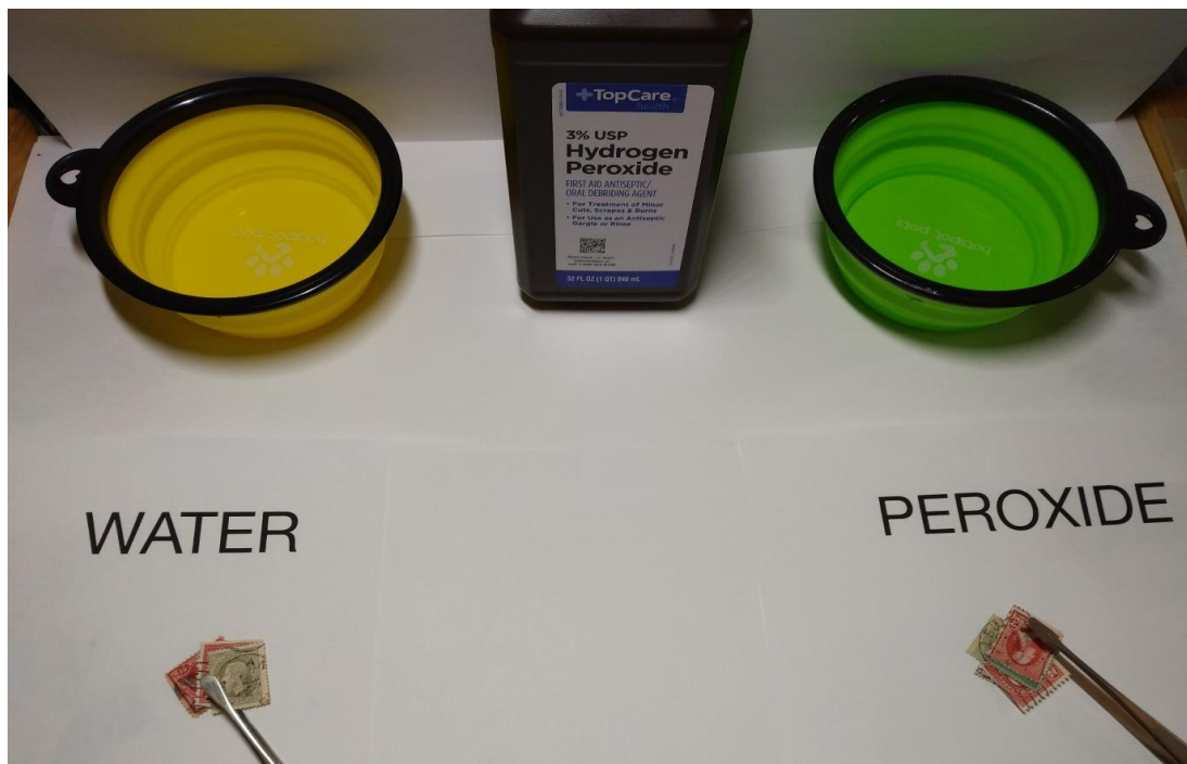
Figure 4: As previously described by Stan, silicone rubber dishes of identical design were used for the study, the one on the left (yellow) for soaking the test specimen in filtered water, and the one on the right (green) for soaking its specimen in full-strength 3% hydrogen peroxide.
