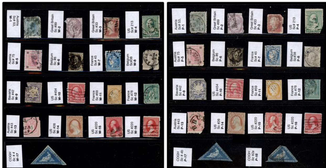
Figure 3: The test specimens, prior to any soaking in this study. Left: This is the Control Group, which would only be exposed to filtered water. These test specimens are numbered W-1 through W-17. Right: This is the Peroxide Group, which would only be exposed to full-strength 3% hydrogen peroxide solution. These test specimens are numbered P-1 through P-18.
